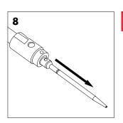
Once the Firing Pin Assembly has been removed from the Guide, slowly release the Trigger Ball and remove it from the Firing Pin Holder.
