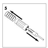
Depress the Reset Spring (NTS5X-11) to collapse the Reset Sleeve. This will loosen the Main Assembly Pin and allow it to be removed from the tool.
