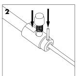
Assemble Firing Pin (NTS101-4) into Firing Pin Holder using the 1/8" Roll Pin (NTS101-8).
