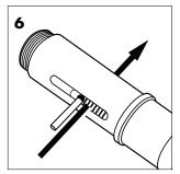
Insert Reset Sleeve into the Trigger Body. Make sure the trigger key on the body aligns properly with the Trigger Ball.
