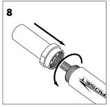
Slide Outer Cover Sleeve over the Trigger Body.
