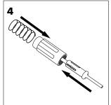
Slide complete Firing Assembly into the Guide while depressing the Trigger Ball until it clicks into the Guide.
